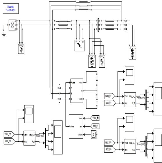
Fig .6, Matlab implementation STATCOM with fuzzy logic controller.
